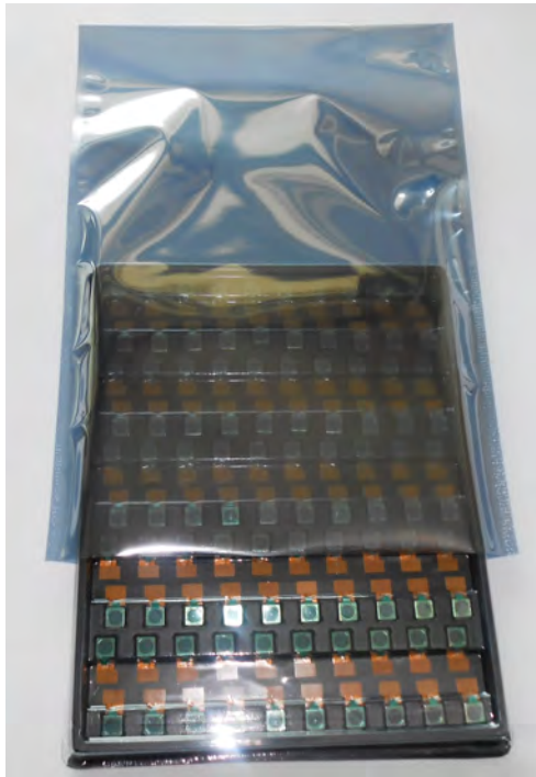
Put Tray into Anti-Static Bag
